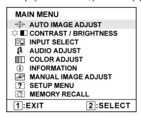
**NOTE:** All OSD menus and adjustment screens disappear automatically after about 15 seconds. This is adjustable through the OSD timeout setting in the setup menu.
